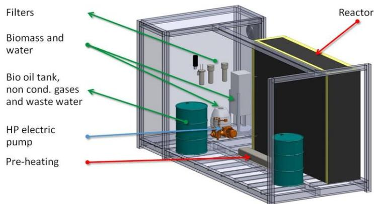
**Figure 2:** Rendering of the plant with shown of main components.
