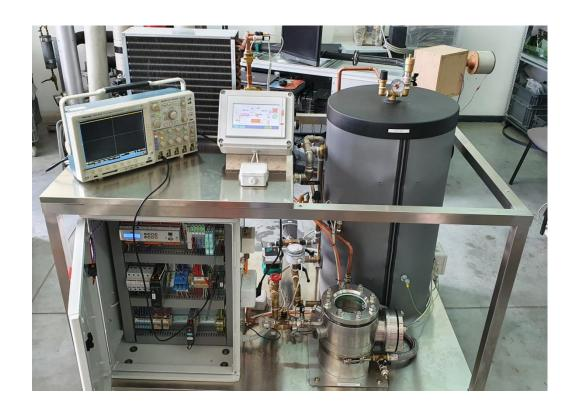
A Test Rig for single phase / condensing / boiling heat exchange between organic fluids (R134a) and brine has been designed and assembled to test different superficial treatments and coatings on metal plates under real operational conditions. Tests will allow to understand critical issues and technological problems before moving to full demonstration scale.
