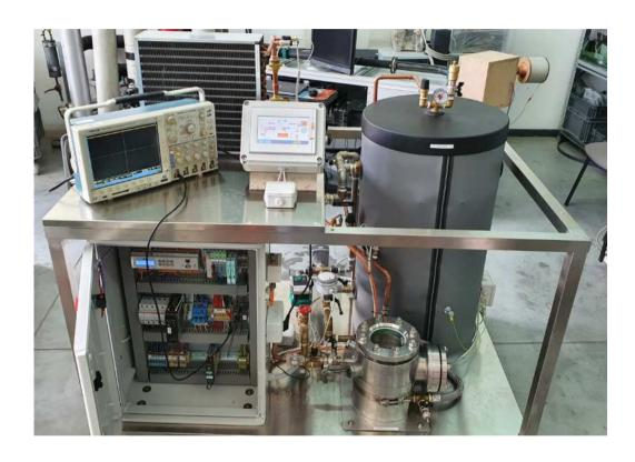
n.3 Test Rigs for single phase / condensing / boiling heat exchange between organic fluids (R134a) and brine has been designed and assembled to test different superficial treatments and coatings on metal plates under real operational conditions. Tests will allow to understand critical issues and technological problems before moving to full demonstration scale.
